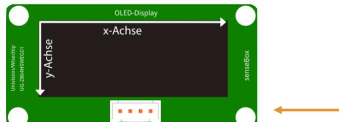
The display has a screen resolution of 128x64 pixels. That means 128 pixels in horizontal direction (x-axis) and 64 pixels in vertical direction (y-axis).
